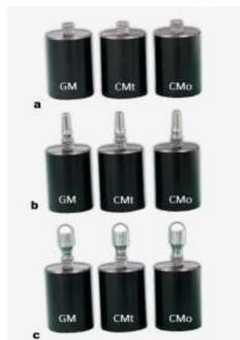
Figure 2. Types of implant-abutment connections used in the study. (a) GM, CMt, and CMo implants were installed in a cylindrical block made of polyacetal; (b) GM prosthetic abutments with a two-piece abutment design featuring a 16° taper, CMt prosthetic abutments with a two-piece abutment design featuring an 11.5° taper, and CMo prosthetic abutments with a one-piece abutment design featuring an 11.5° taper; (c) prosthetic abutments were covered with a semi-spherical rigid body.
