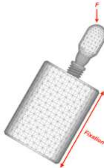
Figure 5. A finite element mesh that simulates the mechanical testing using a vertical load applied to specimens inclined 30 degrees from the vertical axis was developed with Autodesk Inventor Professional 2013 (San Rafael, CA, USA).
