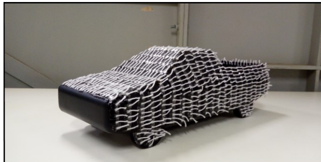
Figure 3: Rounded model setted for the tufts visualization experiment.
