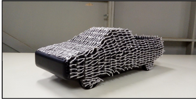
Figure 27: Rounded pickup model set with tufts.
