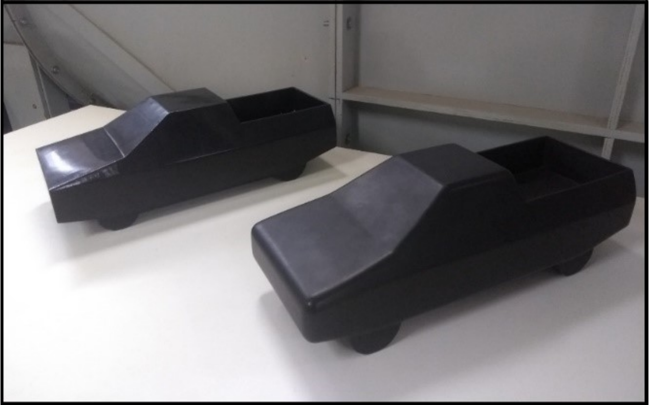
Figure 4: Pickup test models. Left: Flat (Baseline). Right: Rounded.
