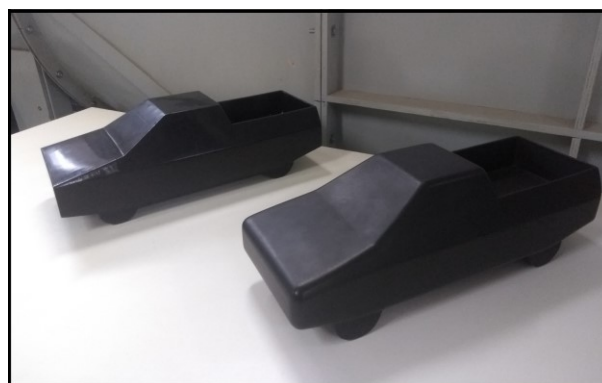
Figure 2: Pickup test models. Right: Flatted. Right: Rounded
