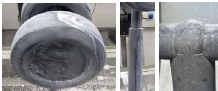
Figure 13. Preliminary flow visualization from China clay technique.
