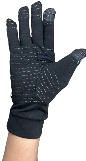
Figure 4.4 – Conductive lines in the first prototype of the HMI.
