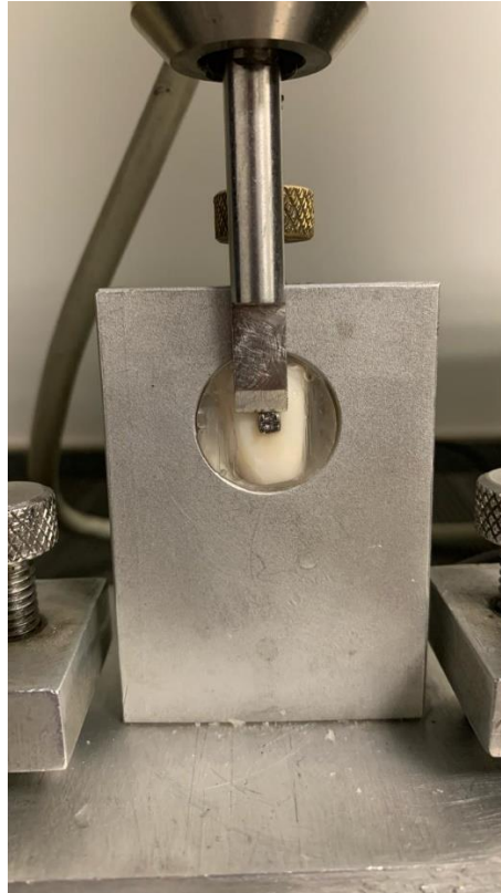
Figure 3. Sample positioned for the shear bond strength test.
