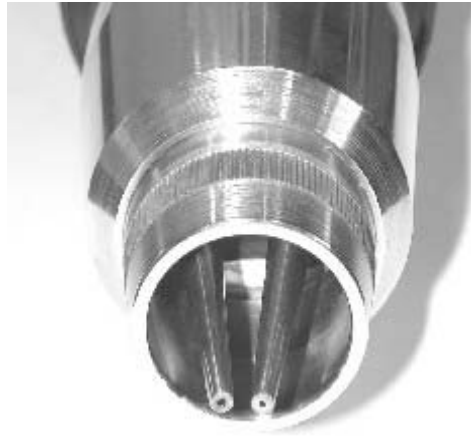
Figure 2.3 - Cranfield Tandem GMAW (WIDGERY; BLACKMAN, 2001)
