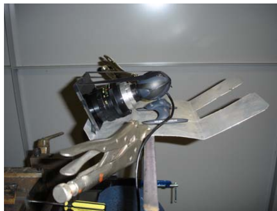
Figure 3.11: Webcam with magnifying lens and filters attached
