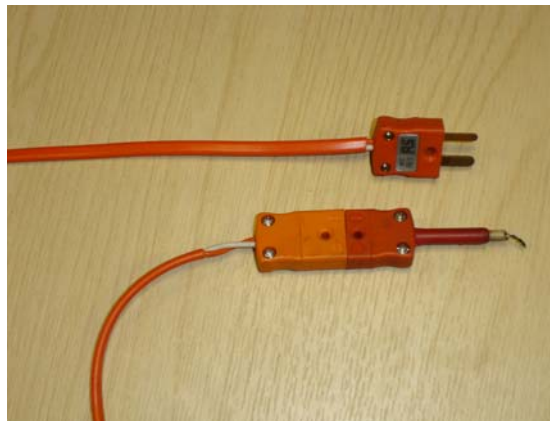
Figure 3.5: Cable for temperature signals
