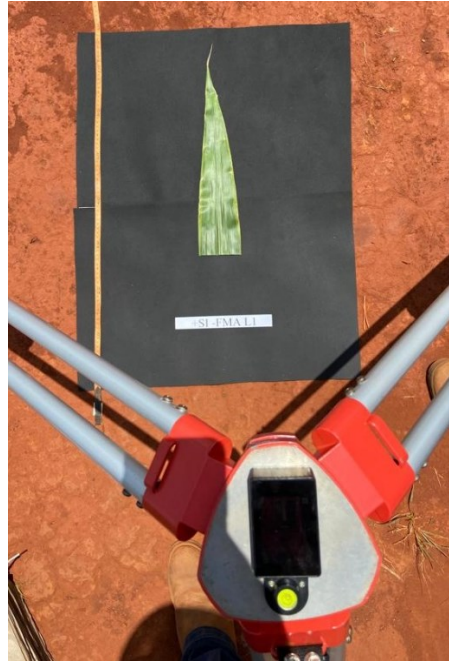
FIGURE 3 Tripod mounted to attach the MAPIR camera (Survey 3) to collect multispectral images on corn leaves.
