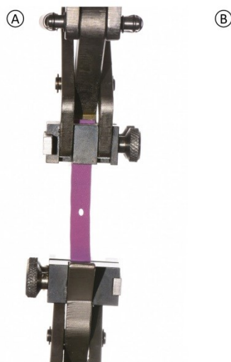
Figure 2. A. Specimen positioned on the clamp before testing. B. Specimen after rupture.
