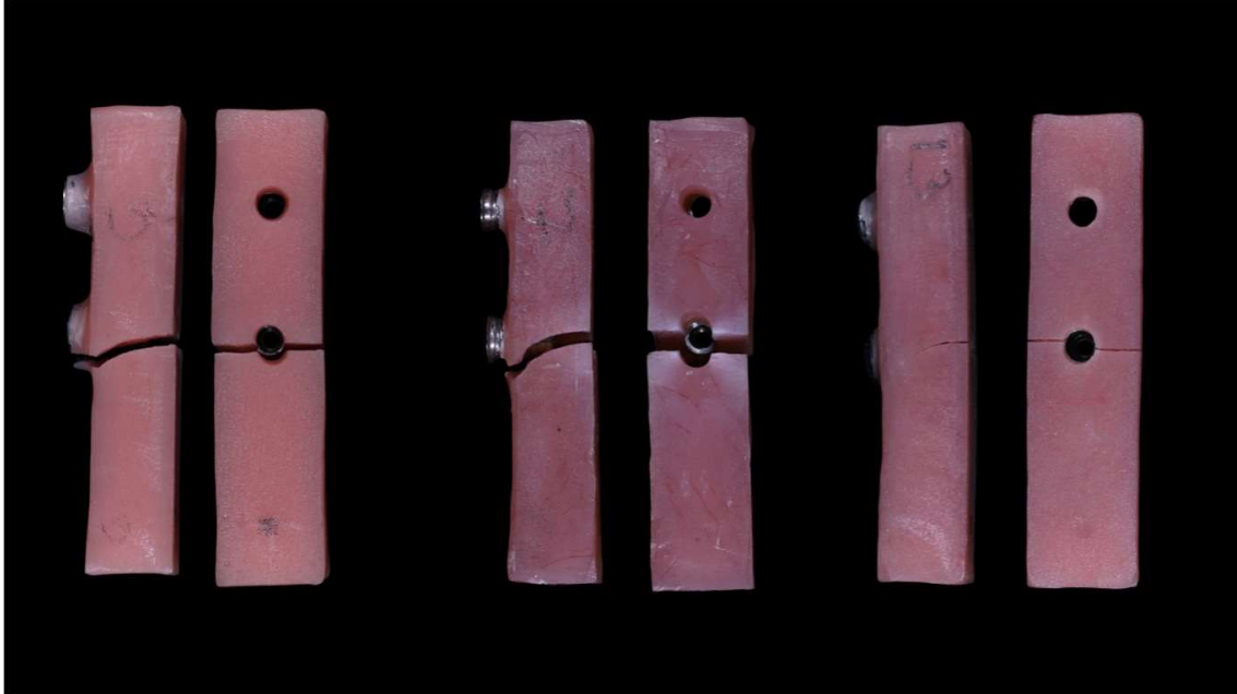
Figure 11- Example of how fractures of the resin samples looked after the tests A - conventionally self-polymerized resins (RA); B- High resistance Thermo-polymerized resin (RD); C-conventionally Thermo-polymerized denture resin (RT)
