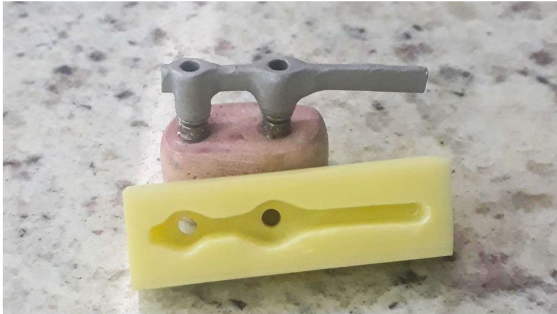
Figure 3 metallic infrastructure cast and finished in nickel chrome, and printed resin bars that will be used as a mold to pour the study resins.
