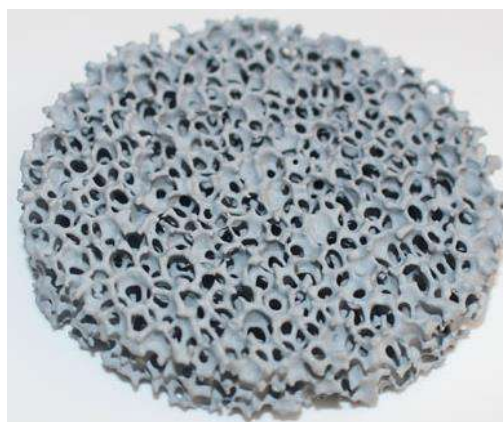
Fig. 3.1. SiC foam used in the catalytic bed during the assisted-microwave pyrolysis experiments.
