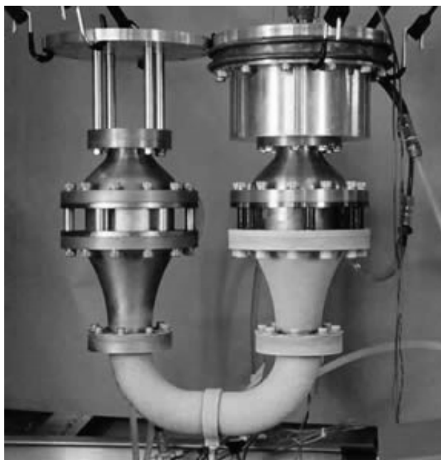
Figura 1.6 – Shipboard Electronics ThermoAcoustic Chiller (SETAC) antes do financiamento apresentado pela Naval Science Assistance Program. (Acousitc, Pennstade Graduate Program).
