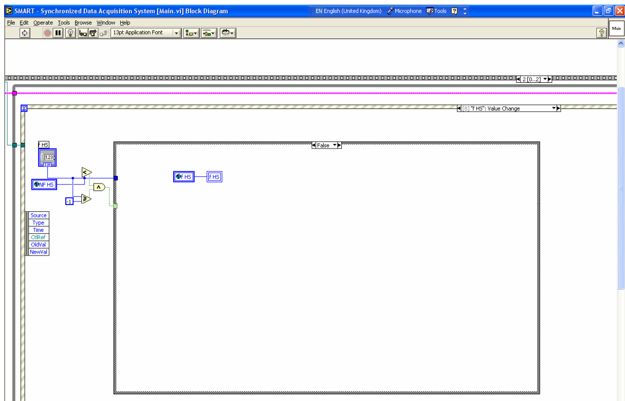
Figure 3.175: Illustration of the code of the event “f HS” that keeps the same HS camera frame if the typed frame is not under the acceptable limits
