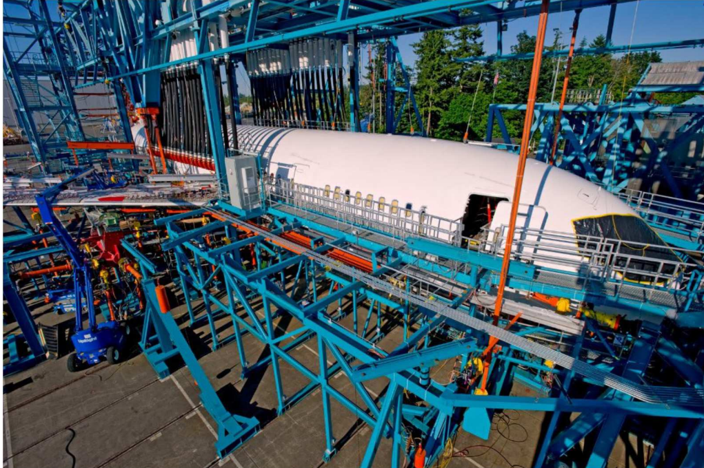
Figure 7 – Structural fatigue test in the fuselage. Source: Aviation Week 2 .
