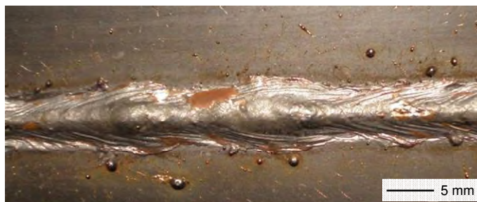
Figure 4.85: Weld bead aspect produced by TandemOptPulse program (no synchronisation between the wires)
