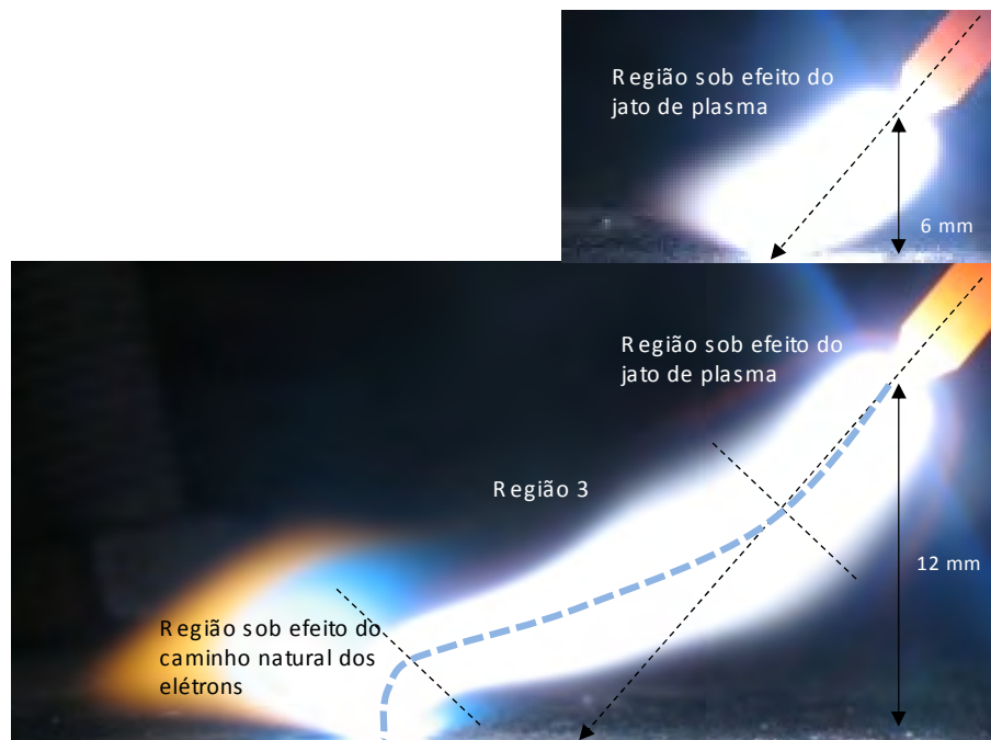
Figure 14: Regions under different effects in GTAW arcs with the same current level and different vertical electrode to work-piece distances
