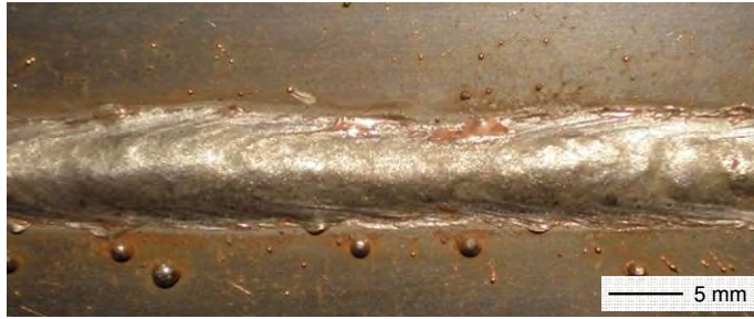
Figure 4.95: Weld bead aspect produced by TandemOptPulse program (synchronisation after state 2 of controlled short-circuit mode and long/low current pulses)
