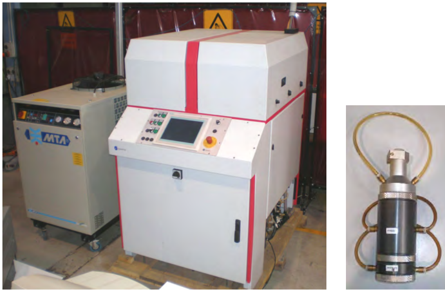
Figure 5.4: Laser system (left hand side) and Laser head (right hand side)
