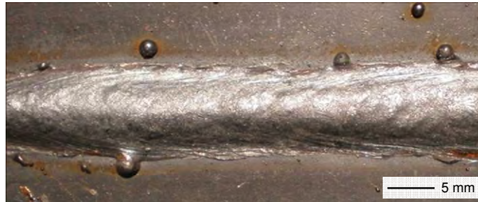
Figure 4.99: Weld bead aspect produced by the TandemOptPulse program with two-steps pulse of current (synchronisation after state 2 of controlled short-circuit mode)
