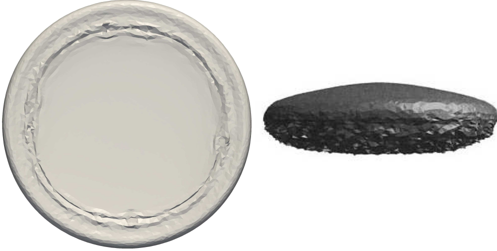
Figure 3.11: Wrinkles at the rear of rising bubbles. Left: Spherical cap, Eo = 40 , M = 0.056 . Simulation carried out in the present Work. Right: Intermediate wobbling + spherical cap, Eo = 10.0 , M = 9.71 \cdot 10^{-12} (ANNALAND; DEEN; KUIPERS, 2006).
