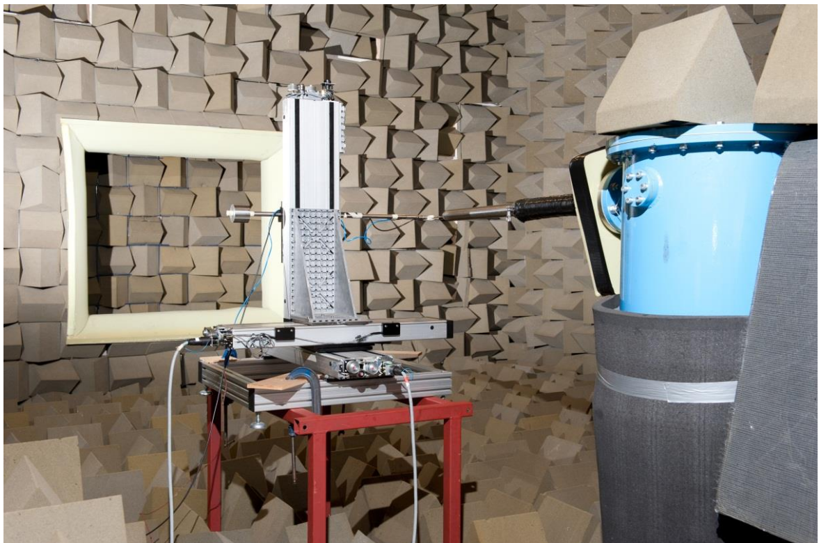
Figure 4.3 – General view of Doak Laboratory with traverse system to hot-wire anemometer and pitot tube measurements.
