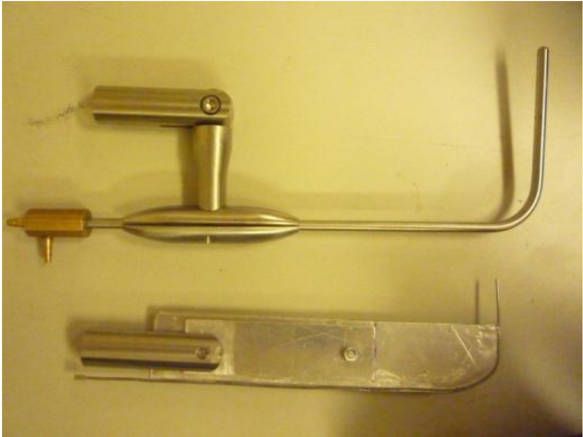
Figure 4.11 - Pitot tube of the micromanometer (above) and pitot tube built during the experiments (below).
