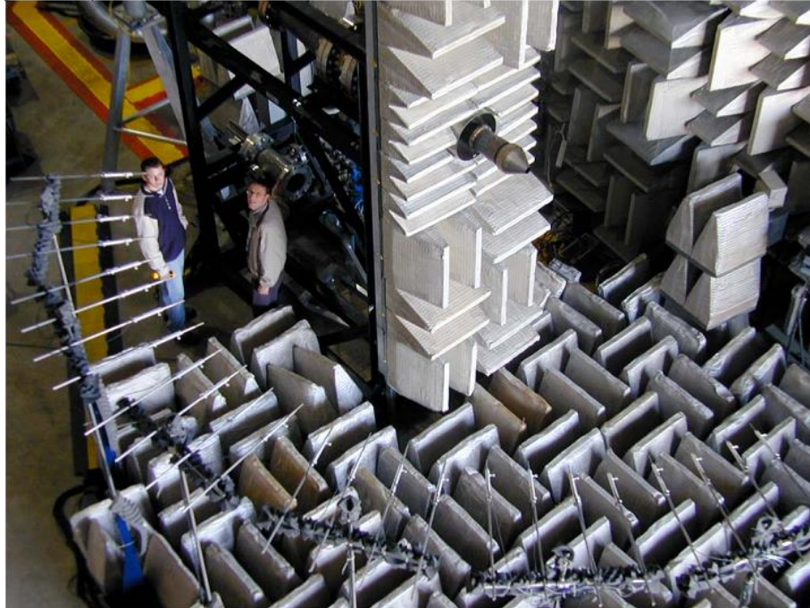
Figure 3.10 – Experimental configuration of SHJAR with microphone array (Brown and Bridges, 2006).
