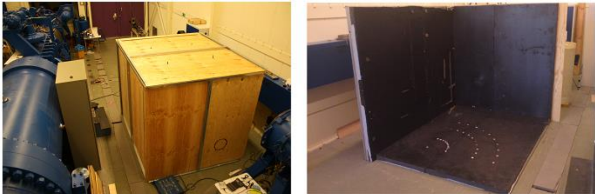
Figure 3.15 – Outside view of the anechoic chamber and inside view with nozzle and microphone (de Boer, 2011).
