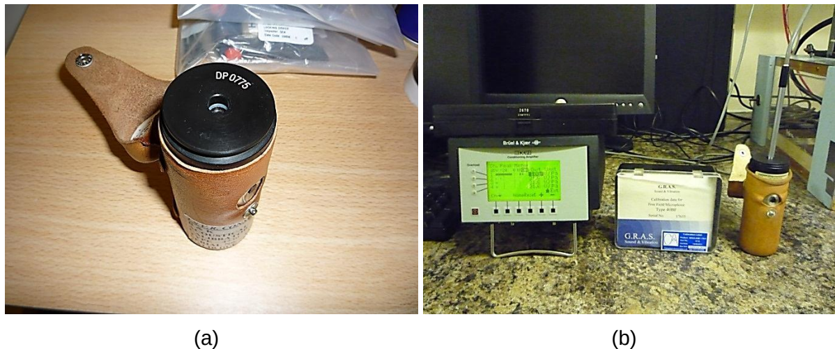
Figure 4.20 – (a) A pistonphone calibrator. (b) Configuration used during microphones calibration.
