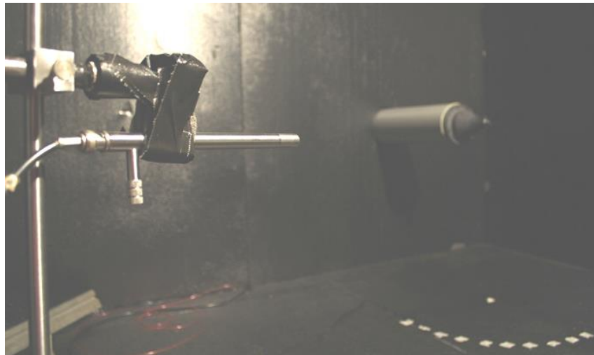
Figure 3.18: Microphone measurements inside the anechoic chamber with r = 1 m and \theta = 90^\circ (de Boer, 2011).
