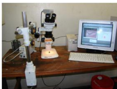
Figura 3.12 - Microscópio SZ6145TR – OLYMPUS e software Image Pro-express (PEREIRA, 2009)
