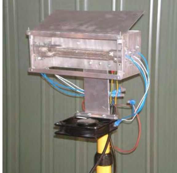
Figure 3.11: Final lamp using 4 halogen bulbs of 1 kW each
