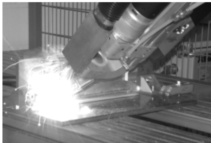
Figure 2.28: Welding operation using Laser - GMAW hybrid process (BWI, 2008)
