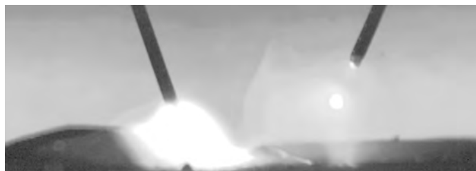
Figure 3.10: Image using 4 halogens bulbs of 1 kW each (as the tungsten filaments were placed to form a big “net” of light, all background was illuminated) (Camera exposure time: 97 \mu s; Lens aperture: 4; Filter: neutral density COKIN P153 grey and red COKIN P3; Correction: gamma 3.5 and saturation 0)
