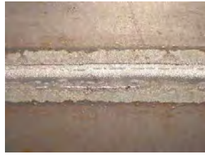
Figure 4.42: Typical root appearance for weld beads of Figure 4.41
