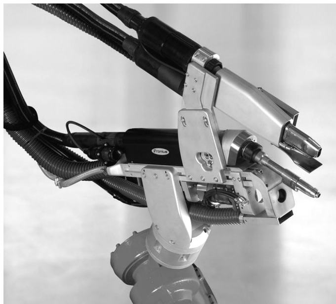
Figure 2.48: Head devised for the Laser - GMAW - tandem GMAW process (FRONIUS, 2008b)
