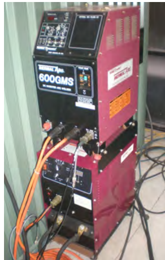
Figure 3.14: Power sources used for the tandem GMAW applications
