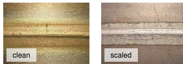
Figure 4.38: Typical appearance of root for weld beads of Figure 4.37
