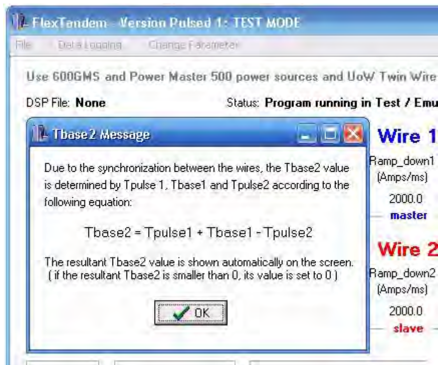
Figure 4.11: Tbase2 Message box in the FlexTandem - Pulsed 1
