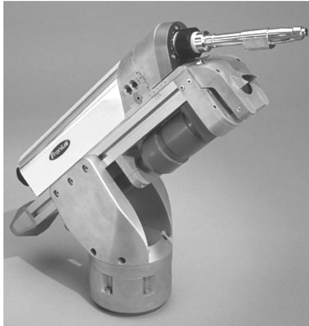
Figure 2.29: Commercial head devised for Laser - GMAW hybrid process (Fronius, 2008a)
