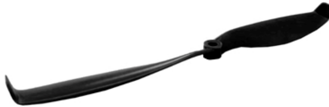
Figure 18 - 10x4.5 Proplet 02 ( h=10\text{mm} ) 18 .
