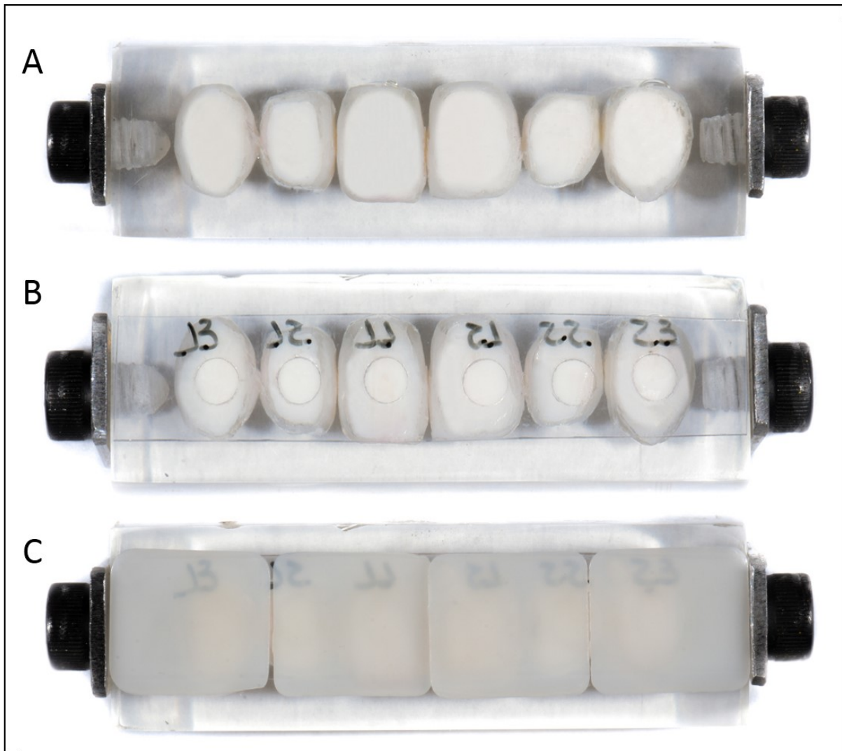
Figure 1. Teeth matrix used on this study. A) Teeth matrix simulating six anterior teeth; B) 0.3-mm thick resin cement matrix with six holes to make luting materials samples; C) 0.5-mm ceramic discs placed above the resin cement matrix.
