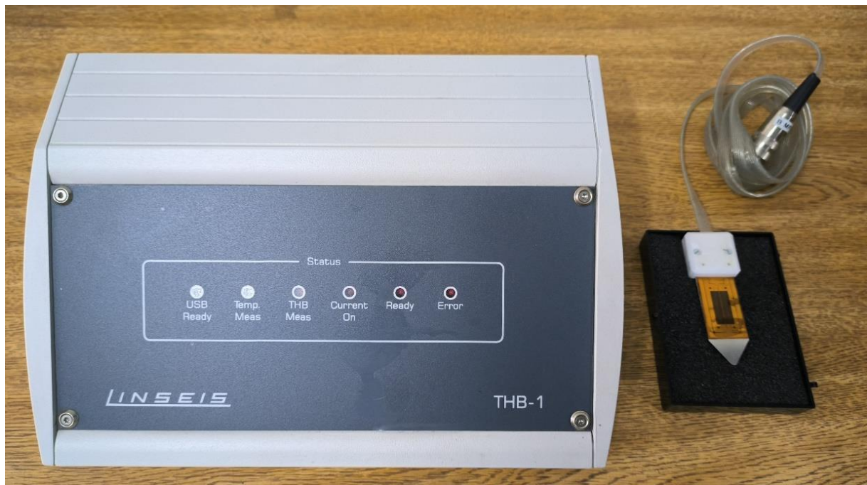
Figure 3.8 – Thermal conductivity meter LINSEIS and THB – 1 sensor. Source: Author's own.
