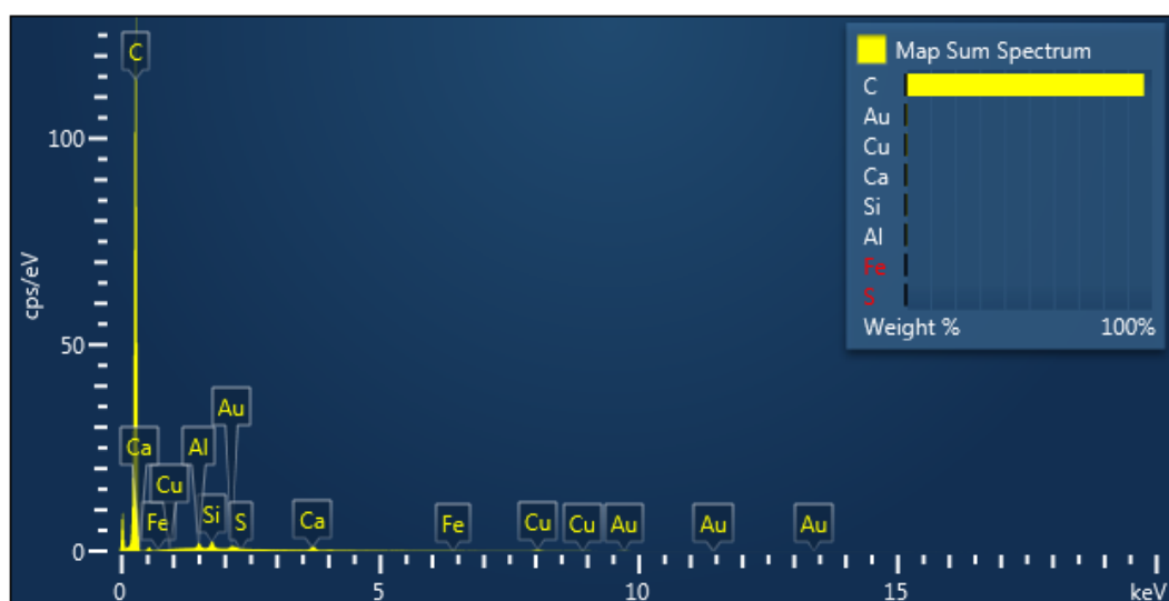
Figure 4A – EDX spectrum for Industrial graphene nanoparticles. Source Author's own.
