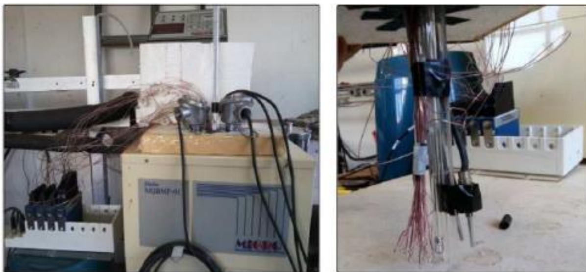
Figure 1B – Calibration process of the thermocouples. Adapted from (Cárdenas Gómez, 2019).
