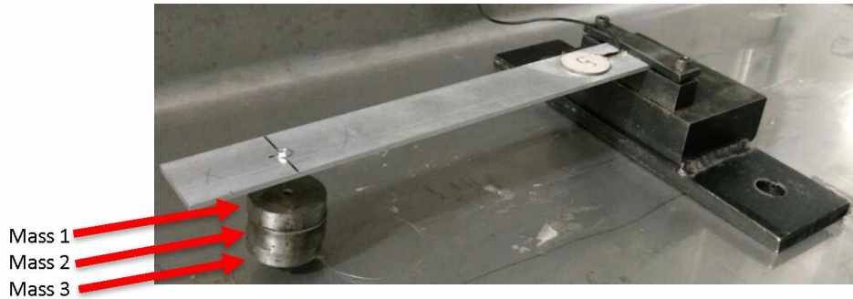
Figure 19 - Clamped beam with the masses 1 + 2 + 3 hanged in the marking (the mark is 152mm away from the PZT)
