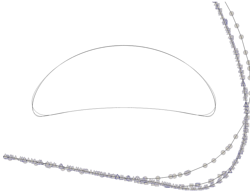
Figure 4.18: Cross section of the terminal bubble shape depending on the Lagrangian edge length, for a fixed Eulerian grid size and varying Lagrangian characteristic length. \circ : \lambda_\xi = 1 . \square : \lambda_\xi = 2 . \triangle : \lambda_\xi = 4 .
