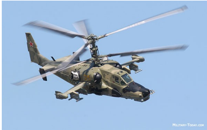
Figura 10: Helicóptero com rotor coaxial (Fonte: https://www.quora.com/Why-coaxial-helicopter-rotor-blades-are-so-uncommon )
