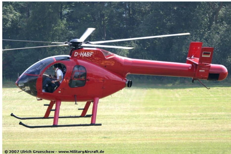
Figura 12: Helicóptero do tipo notar - MD 520-n (Fonte: https://www.militaryaircraft.de/pictures/civilian/helicopter/MD-500/MD-500.html )
