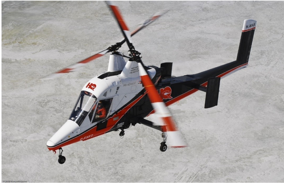
Figura 9: Helicóptero com rotor contra-rotativo - Kaman K-Max (Fonte: http://vantvirtual.blogspot.com/2013/02/helice-ou-rotor-de-helicoptero.html )
