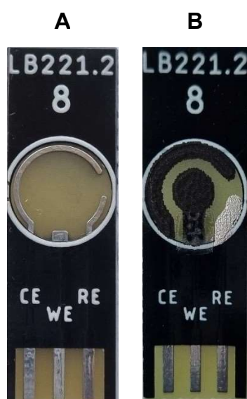
Figure S 2: CPCB-E electrode before (A) and after (B) the ink deposition.
