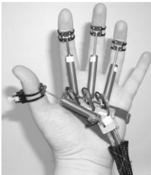
Figura 2.11. Rutgers Master II-ND (Bouzit et al., 2002).
