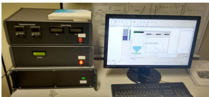
Figuras 18 e 19 - Aparelho nanodurômetro ASMEC – Advanced Surface Mechanics GmbH (Grupo Zwick Roell, Oliver & Pharr, 2004, Alemanha)
