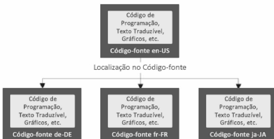
Figure 33.3 - When localization is performed in the source code, it is necessary to maintain a separate set of code for each target locale plus one set for the domestic market
