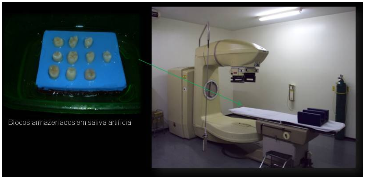
Figura 2: Equipamento de telecobaltoterapia modelo Theraton Phoenix Cobalt 60 Radiotherapy Treatment Unit
