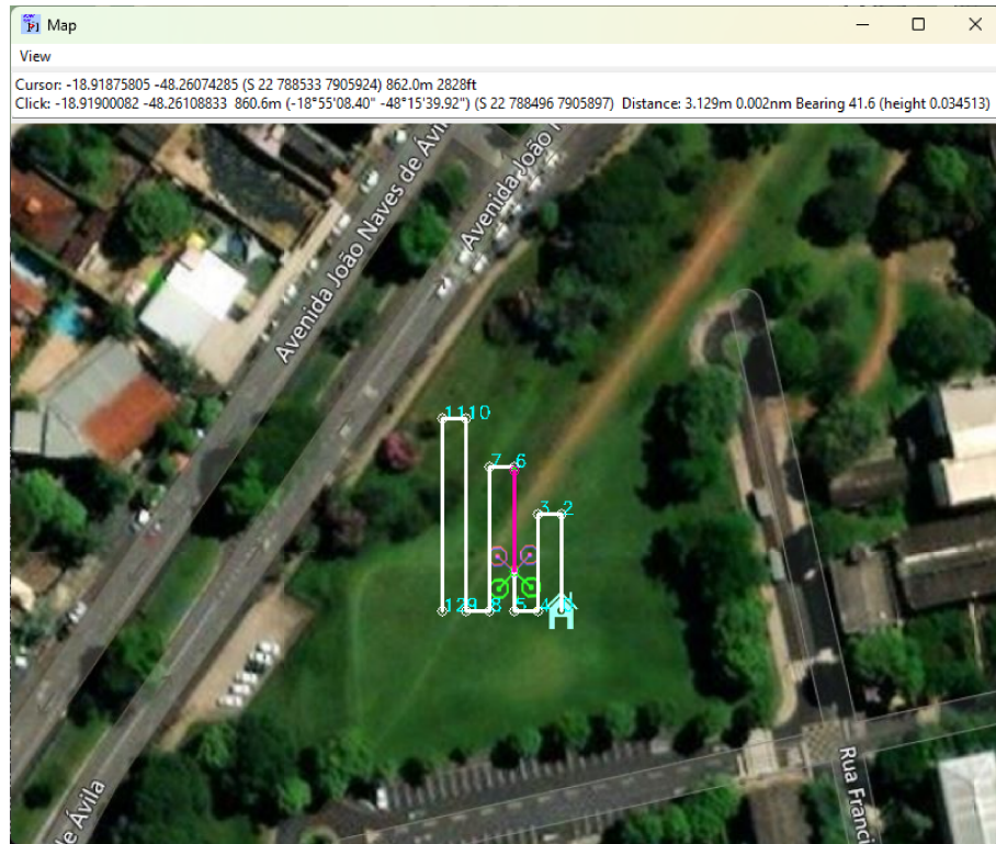
Figure 31 – Visualization of the test trajectory presented in a SITL window.
