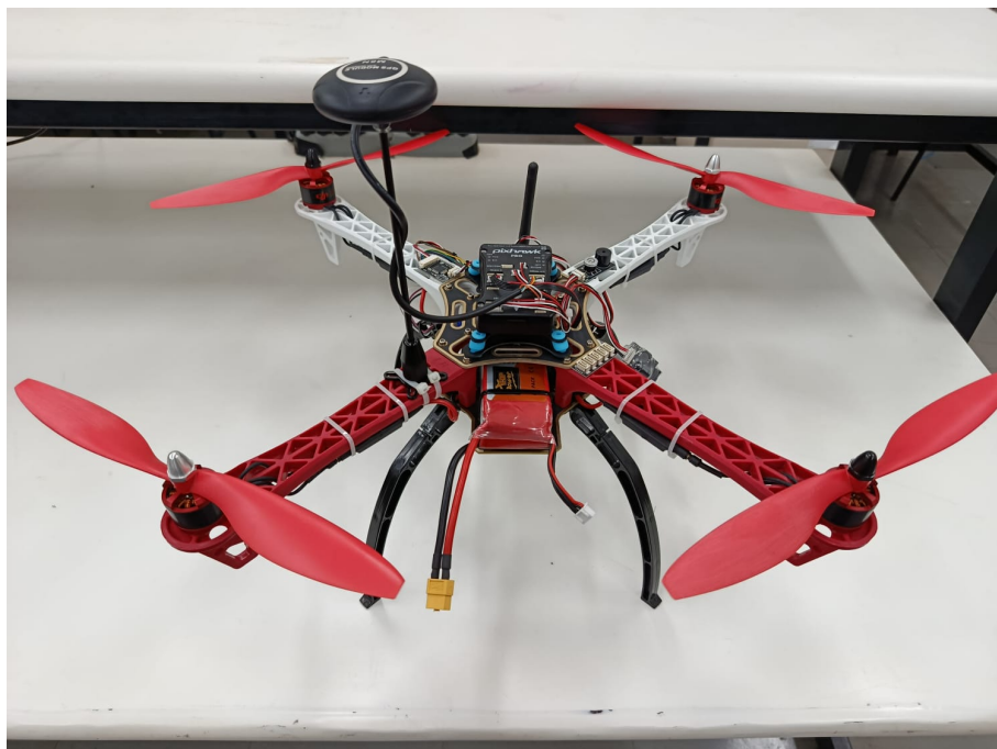
Figure 28 – UAV prototype used for the project The vehicle is based on the F450 frame and the Pixhawk 2.4.8 controller.
