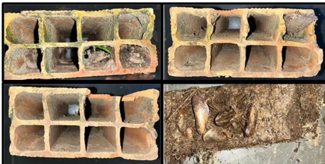
Figure 3. Bricks recovered after 90 days of submersion.
