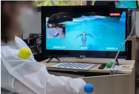
Fig. 13. Pilot test of the proposed exergame system with a post-stroke patient. The game runs on a smartphone and is mirrored on a television screen. Colored markers on the arm enable real-time 3D tracking using the smartphone's webcam.
