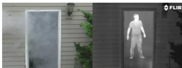
Figure 6 – Example of infrared camera usage for identifying people in thick smoke, showing how optical thickness can be different for different regions of the electromagnetic spectrum. Figure issued by specialty camera manufacturer FLIR and taken from Bhowmik and Sen (2016).
