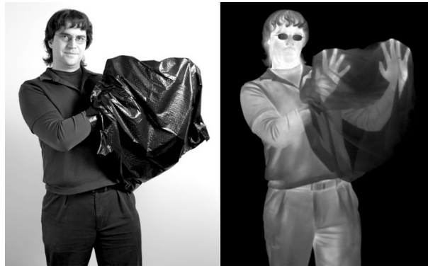
Figure 5 – The spectral properties of materials change spectrally. The left picture is taken from a normal camera, while the right is taken with an infrared camera. One can observe the man's hands through the plastic bag on the right picture, but not on the left. Similarly, his glasses are opaque in the infrared picture. Figure taken by NASA and adapted from Hurt (2025).
