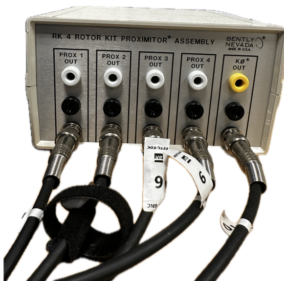
(a) Conjunto Proximitor Bently Nevada
