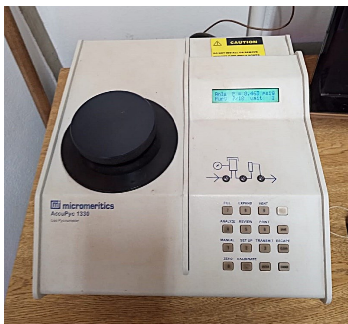
Figura 3.2 – Picnômetro Micromeritics AccuPyc 1330.
