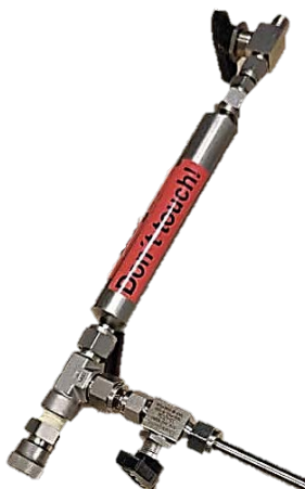
FIGURE 12. Gas mouse used to store the gases collected post reaction.
