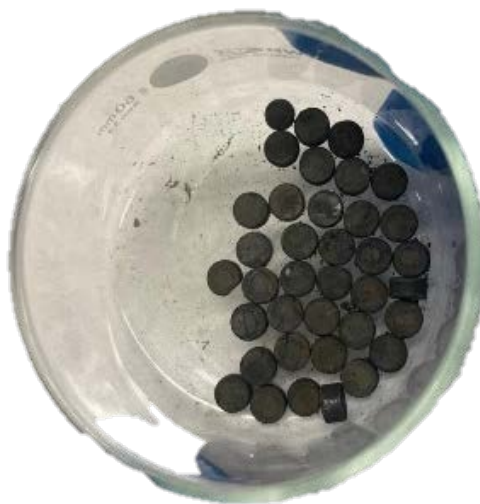
FIGURE 3. \text{Nb}_2\text{O}_5 Pellets Impregnated with 5%Ru.
