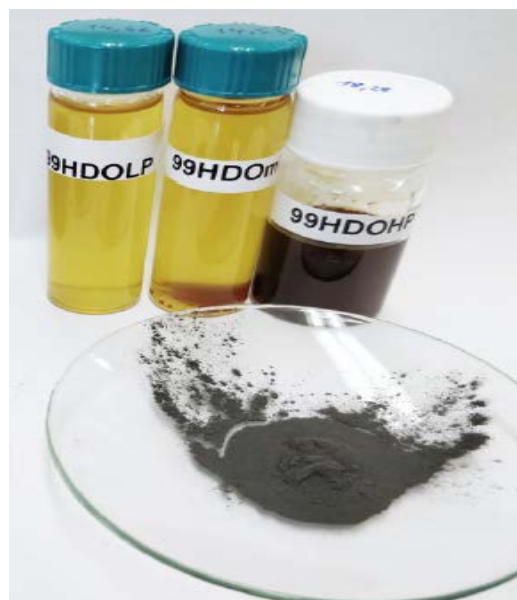
FIGURE 10. Product separation due to Centrifugation. Light Aqueous Phase on the left, oil phase on the right and in the bottom is the solid Residue.
