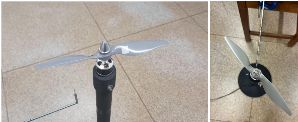
Figure 4. Hot wire anemometer positioned in the propeller wake.
