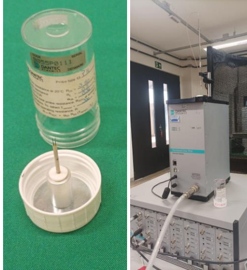
Figure 5. Hot wire anemometer probe (1D) and the calibration system.
