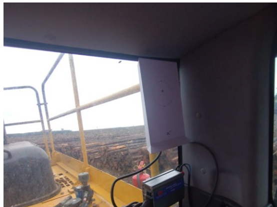
Figura 17 – Router Starlink na cabine do Feller.
