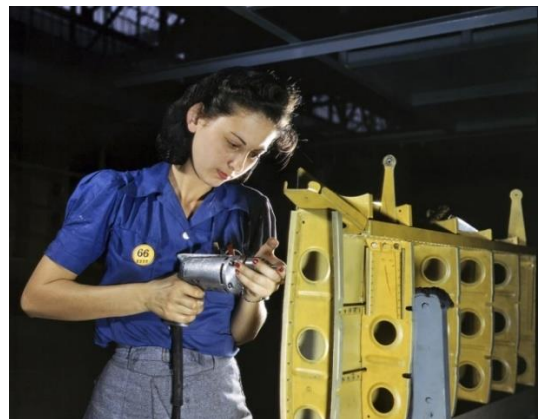
Imagem 58: Palmer, Working on the horizontal stabilizer of a “Vengeance” dive bomber at the Consolidated-Vultee plant in Nashville.
