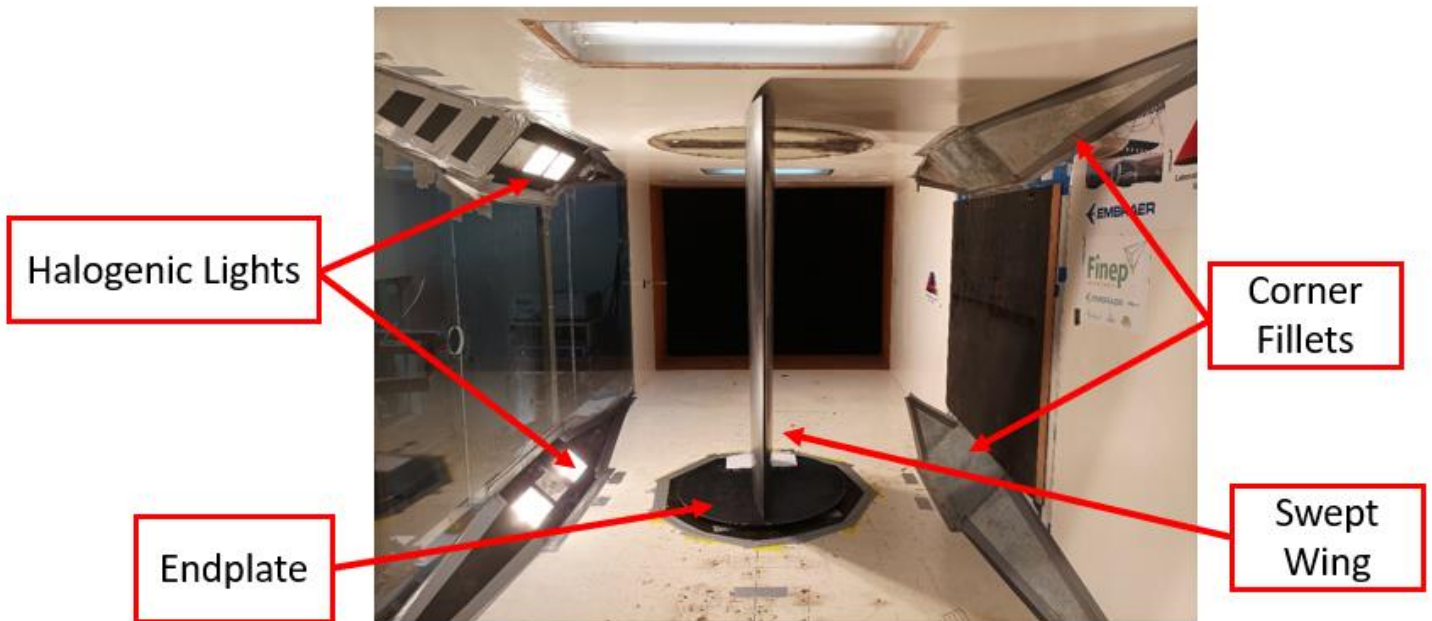
Figure 4.13: Allogeneic lights and corner vanes installation into the wind tunnel test section.
