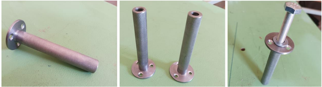
Figure 4.7: Attachment screws used for the wing model attachment to the endplate.
