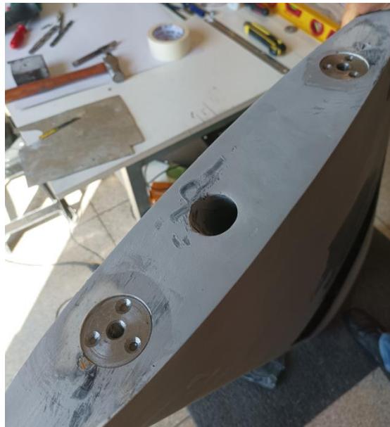
Figure 4.6: Swept wing model basis with fixation discs attached.
