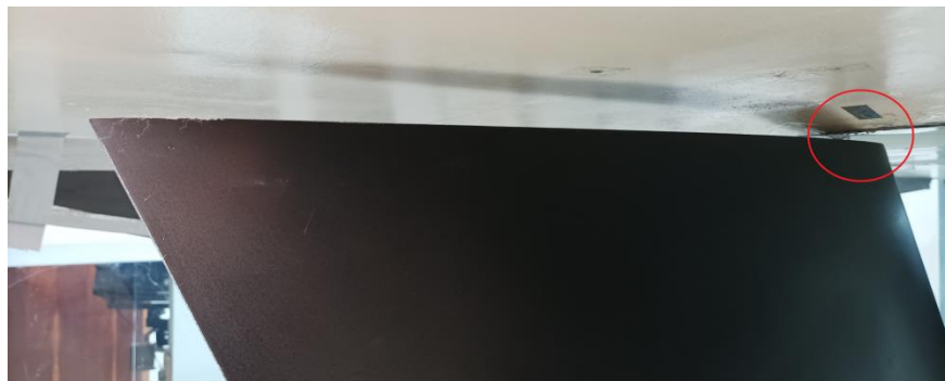
Figure 4.4: Gap between the swept wing model and the wind tunnel superior wall.
