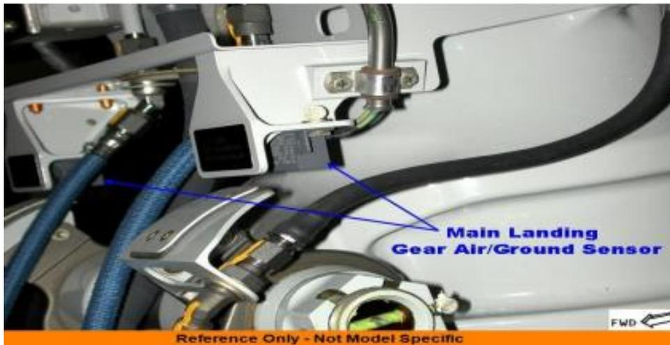
Figura 19: sensor Air/ground (BOEING, 2020)
