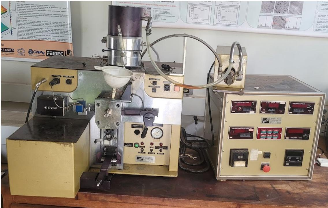
Figura 3.1 - Falex® Block-on-Ring test machine.
