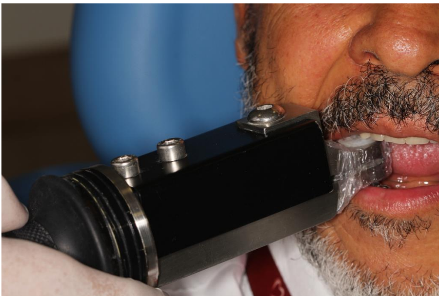
Figure 6 – Measurement of the maximum bite force with the Bite Force Transducer (Gnatodynamometer).
