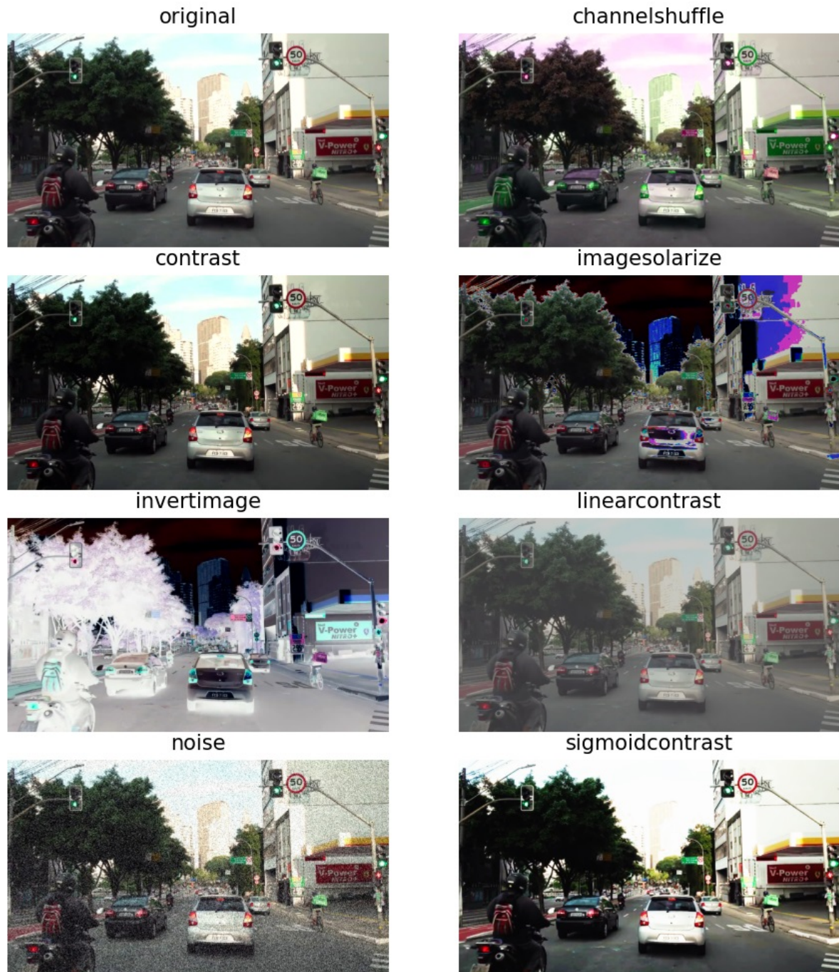
Figure 33 – Example of the augmentation methods on one image. Source: (The authors, 2023).
