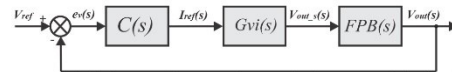
Fig. 12. Block diagram of the approximate equivalent system of the closed-loop BTHR converter.
