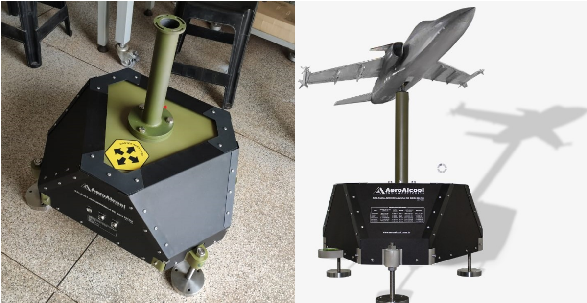
Figure 3.4 – Six-component external wind tunnel balance
