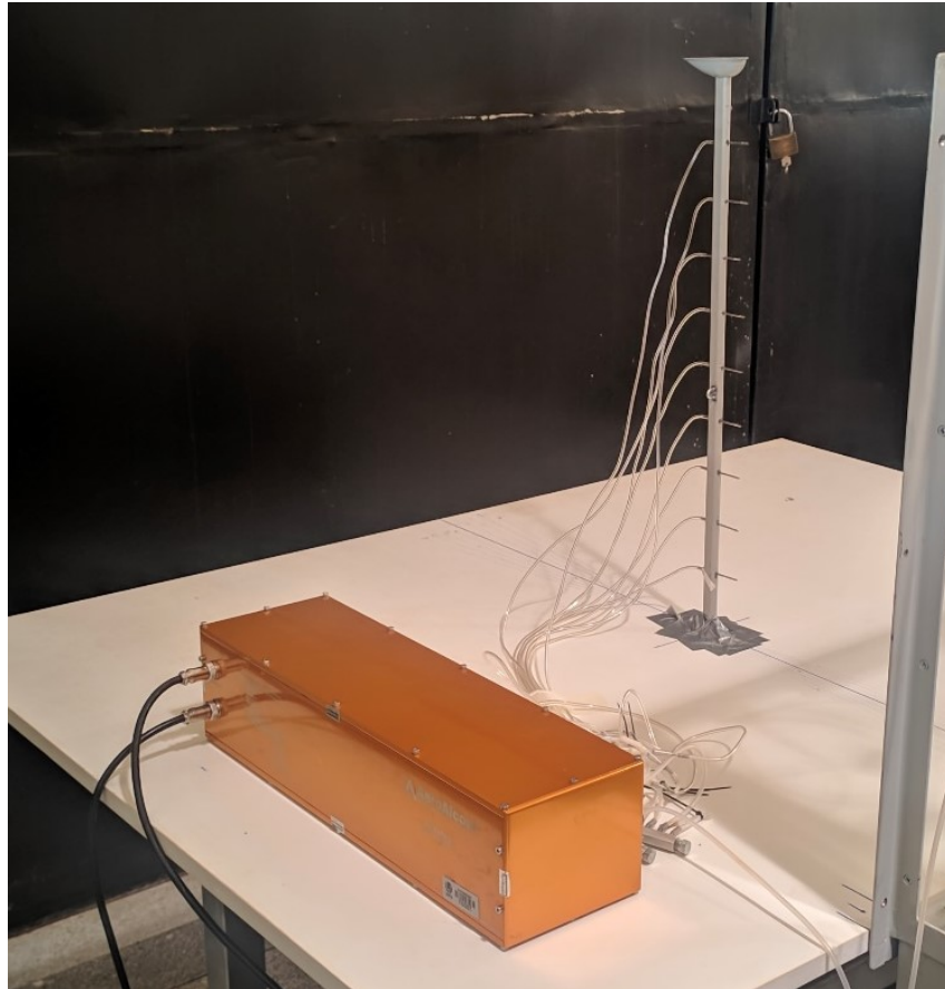
Figure 3.6 – Rake probe with pressure taps
