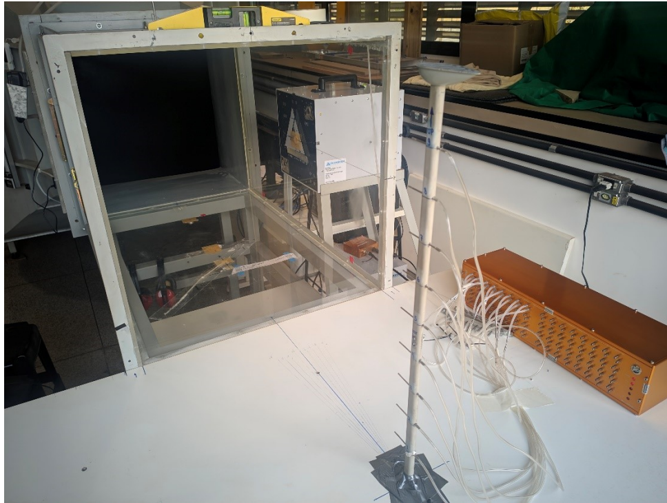
Figure 3.3 - Wind tunnel test section with rake probe
