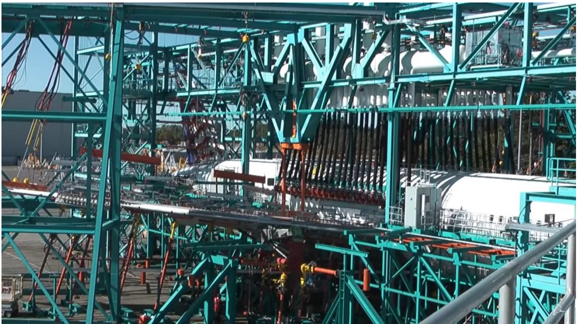
Figura 25 - Ensaio de fadiga full scale do Boeing 787 Dreamliner. (Boeing, 2009)
