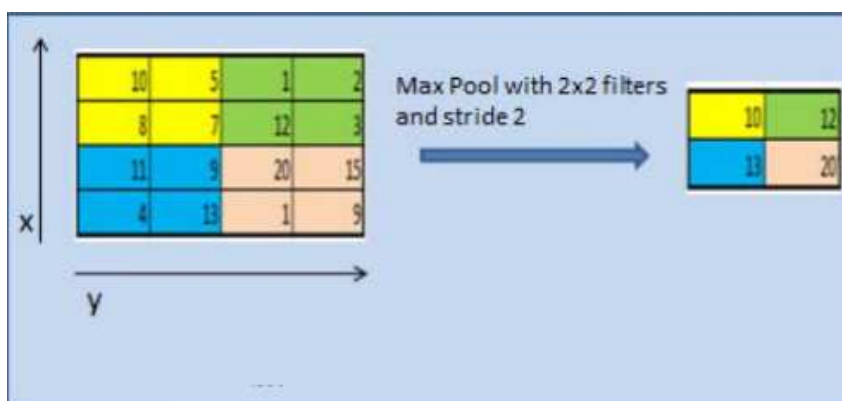
Figure 4 – Example of a max pooling operation in a 4x4 input.
