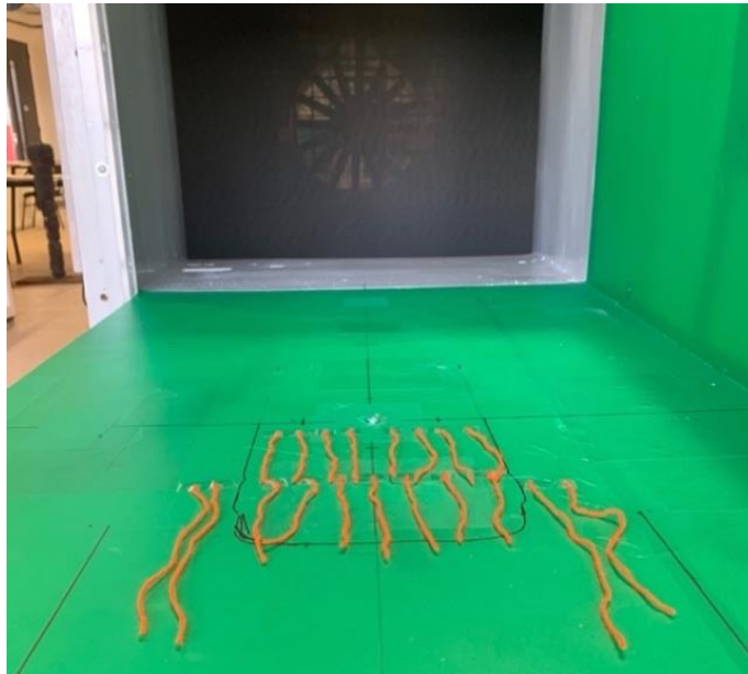
Figure 4.30 – Wall tufts at the ground of wind tunnel test section
