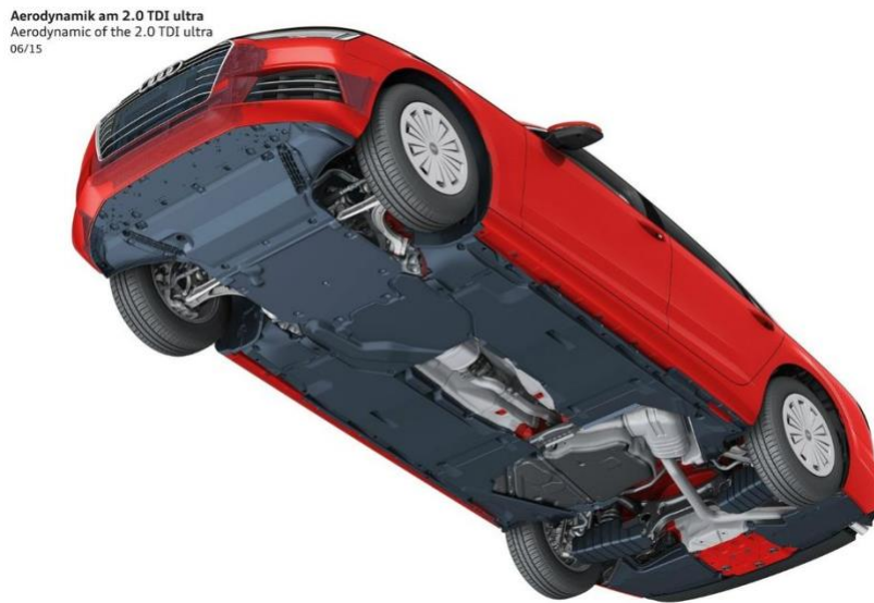
Figure 1.18 – 2015 Audi A4 underbody panels
