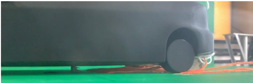
Figure 5.21 – Ground tufts lifted for 6-degree diffuser
