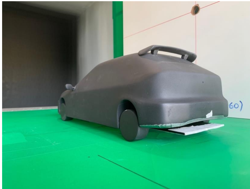
Figure 4.22 – 0-degree diffuser configuration
