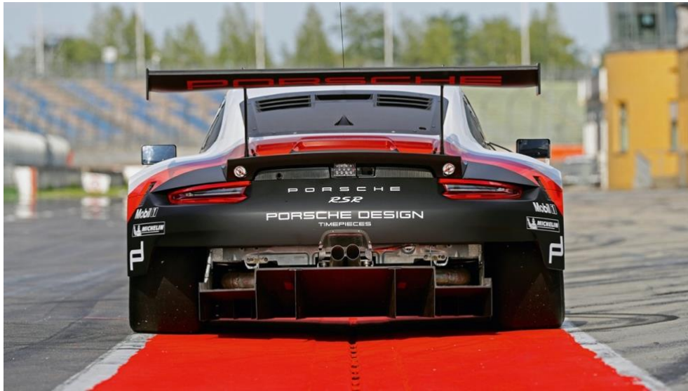
Figure 1.15 – 2017 Porsche 911 RSR rear diffuser
