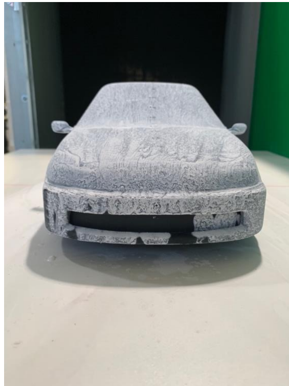
Figure 4.32 – Painted model for flow visualization
