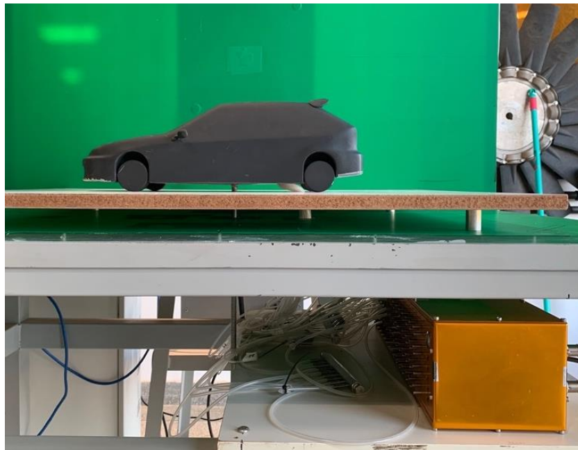
Figure 4.27 – Baseline model pressure field determination
