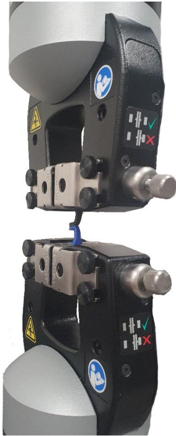
Figure 3. Laminate bond strength test using a universal test machine with a pneumatic gripping for fixation of the EVA specimen.
